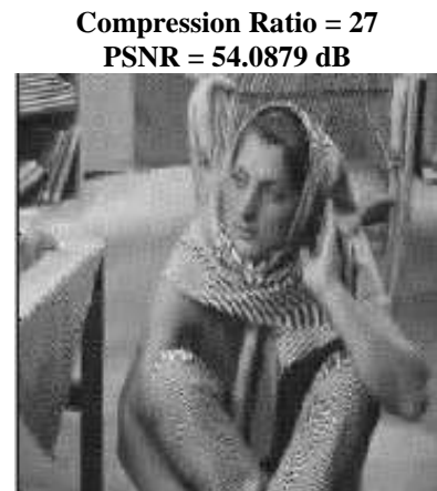
Figure 5.2.118 Compressed image with P = 40 using Huffman Encoding
