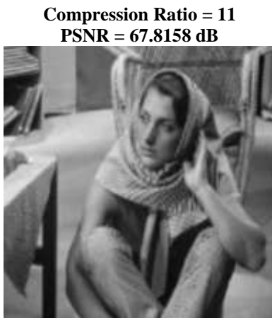
Figure 5.2.27 Compressed image with P =10 using Arithmetic Encoding
